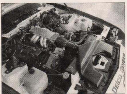
Under its hood, the race car's 305 small-block looks just as it came from the production line. However, "race preparations" include blueprinting the engine and injector to maximize performance and reliability. This particular engine was raced for 70 hours using Mobil 1 oil. When rebuilt, only the seals and bearings were replaced, though still in excellent condition.
