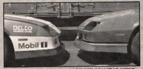
Refinements in the suspension include a lower oversil ride height of about 1.00 inch, created by carefully selecting the shortest springs from a particular batch, as these vary from one to another. The shocks and anti-roll bars are also changed to sull various racing circuits throughout the season.
