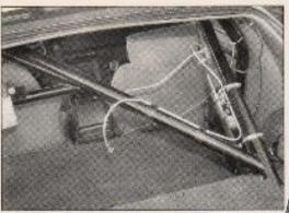
The right rear upright support of the rollcage is also the mounting point for the Halon fire extinguisher. Its nozzles are located across the interior.
